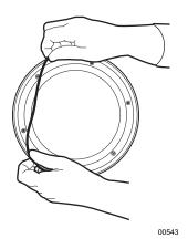
a. Lightly apply O-ring lubricant to the O-ring. Install the
